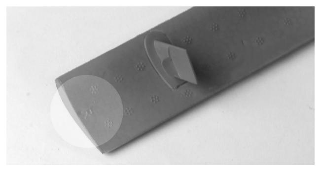
2. Note the slat locating marks at the leading edge of the wing. These have been molded into the wing for your convenience in installing the slats. Use a #11 hobby knife to cut a 1mm (0.04-inch) slot at each of these marks. Test fit the slat as needed to confirm proper fitment.
