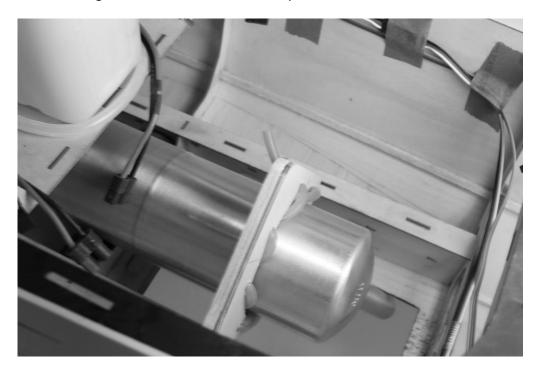
10. Assemble your canister mount (if required), and slide it over the rear of the canister (while the canister is in the fuselage). Note that the canister will not fit into the fuselage if you put the mount over the canister outside of the fuselage.
