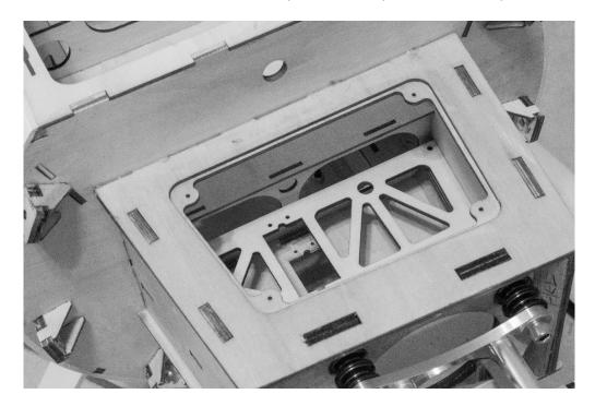
1. When using the DA-70 with the recommended MTW canister, you will need to install the included servo mounting tray into the airplane. Follow the steps the main manual outlines for installing the servo tray. Be sure the hole for the servo is on the right side of the aircraft (if viewing as the pilot).
