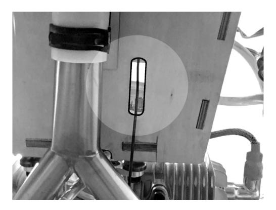
6. Using a rotary tool, cut a small notch in the bottom of the motor box to allow the linkage to pass through and reach the servo. Keep this notch as small as possible, while still allowing the linkage to move freely. Test the servo with the linkage attached to be sure everything moves free with no interference. Secure the linkage in the quick connect as shown in the manual.
