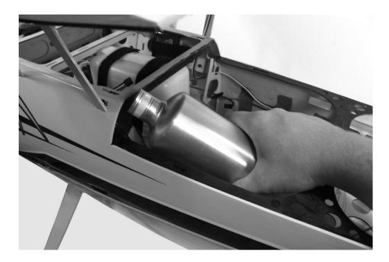
9. The canister is a tight fit into the fuselage, but will fit. Insert the exhaust side of the canister under the radio tray, and to one side of the fuselage. The side of the canister that goes towards the nose of the airplane will be on the opposite side of the fuselage, and pass just in front of the hole location for the canopy dowels. If using the Aura 8 AFCS, it is best to install the canister before installing the Aura brace. Reference the photo above.
