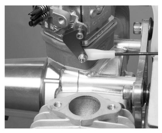
4. Install the white ball link to the included throttle linkage, and secure the linkage to the throttle arm on the engine using the hardware shown in the main manual.
