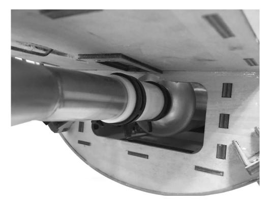
8. Install the plastic coupler onto your header, and install the clamp at this time. Now is also a good time to slide the canister clamp onto the coupler to prepare it to receive the canister.
